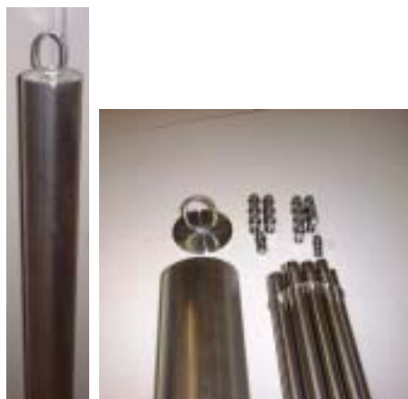
Figure 1: Canister for non-intact and individual fuel rods
