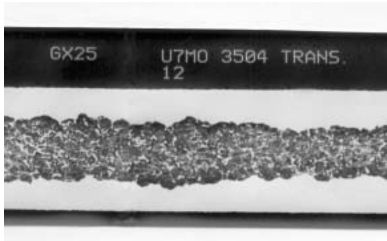
Fig. 1 : Metallographic longitudinal section of as-fabricated UMo sibling fuel plate (U7MQ3504)
