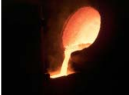
Figure 2: Casting of the first CASTOR BR3®.
