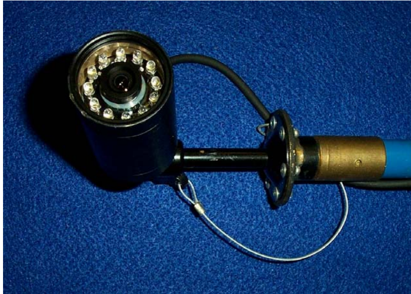
Fig. 2. The camera assembly showing the array of 12 LEDs, the tip of the deployment tool and camera safety cable (note buffer rods not shown).
