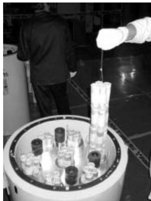
Fig.1 Design of TWR-S fuel assembly and placement of the TWR-S slugs into the TK-S16 containers
