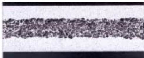
New high density 73 % enriched plate
